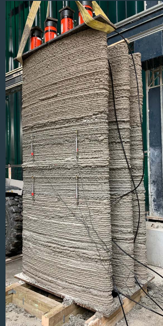
Advanced and Additive Manufacturing Experiments on 3D printed concrete fin walls
