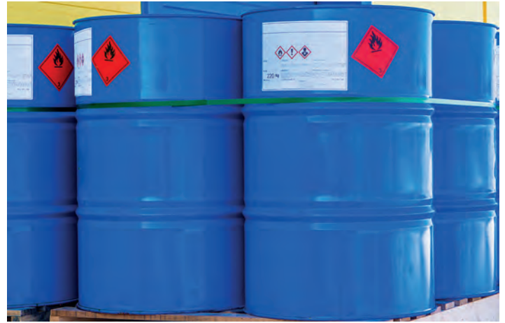
Figure 1 Barrels marked with human health hazard, danger and flammable warning symbols
