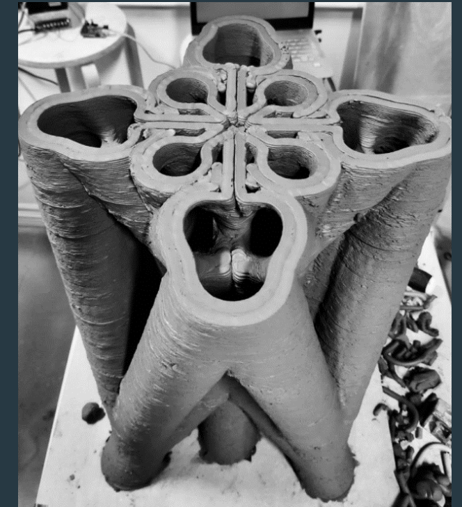
SUTD Additive Manufacturing A 3D-printed clay mold used to cast concrete in. Once the concrete is cured, the clay was washed off to reveal an elegant sculpted concrete structure
