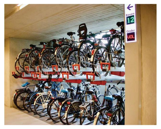
Figure 17: The Utrecht Stationsstalling with automated data collection and electric light signs to indicate vacant spaces (Source: https://www.welovecycling.com/wide/2019/09/30/worlds-biggest-cycling-garage-opens-obvious-ly-in-the-netherlands/)
